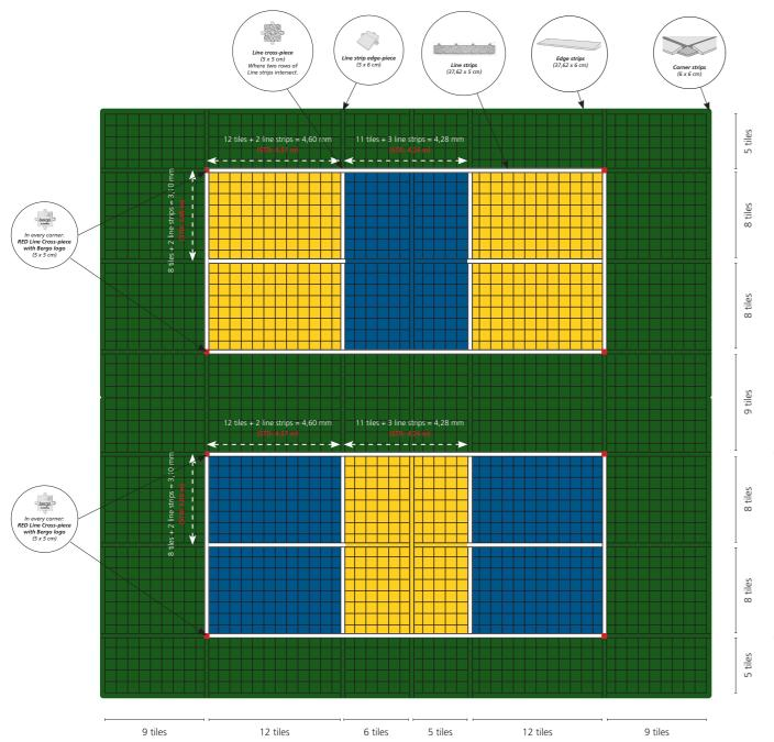
16 tiles + 3 rows of line strips = 6,17 m Standard size according to (IFP) is 6,10 m 12 tiles 12 tiles 6 tiles 5 tiles 12 tiles 12 tiles 12 tiles 13 tiles + 5 rows of line strips = 13,42 m Standard size according to (IFP) is 13,41 m
